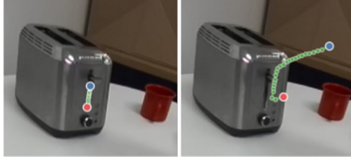
Figure 3: Object trajectory vs. gripper heuristics. Prior datasets often use hand or gripper trajectories as motion heuristics, but these can involve unwanted pre-contact motion (right). We track the object motion itself, which is more straightforward (left).
